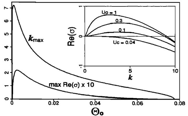
Fig. 2. Inset: dimensionless growth rate  $Re(\sigma)$  versus wavenumber  $k$  (for dimensionless temperature  $\bar{\Theta}_o = 10^{-2}$  and various dimensionless horizontal velocities  $\bar{U}_o$ ) for the theoretical model. Outer figure: maximum growth rate  $Re(\sigma)$  and corresponding wavenumber  $k_{max}$  (i.e., the  $k$  at which  $Re(\sigma)$  is maximum) versus temperature  $\bar{\Theta}_o$  for  $\bar{U}_o = 0.1$ . The viscosity ratio is  $\eta_c/\eta_h = 1000$  in both figures.
