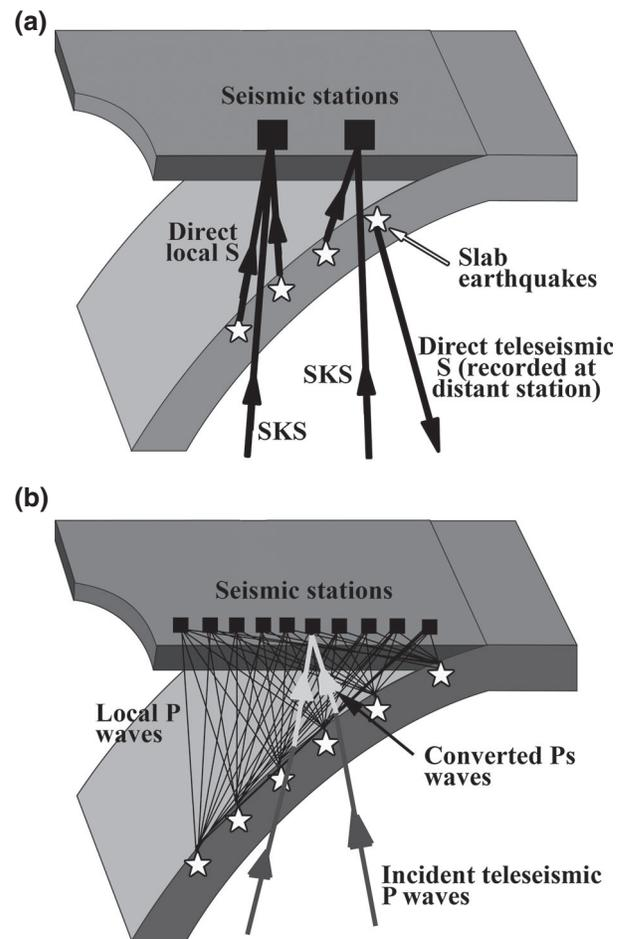
**Figure 1.** (a) Sketch of seismic raypaths commonly used in shear wave splitting studies to probe different parts of subduction systems, including local *S* phases, *SKS* phases, and direct teleseismic *S*, after Long and Silver [2009]. (b) Sketch of seismic raypaths commonly used in receiver function and *P* tomography studies to probe anisotropy in the mantle wedge and slab.
