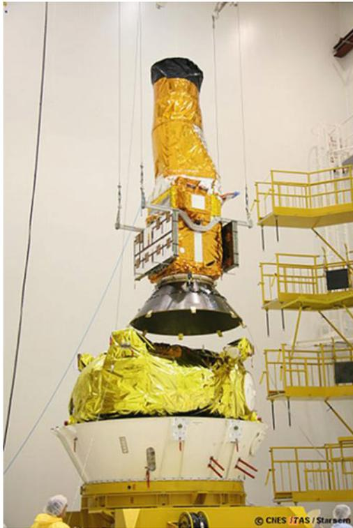
**CoRoT Satellite.** Figure 1 The CoRoT satellite during its integration onto the Soyouz launcher
