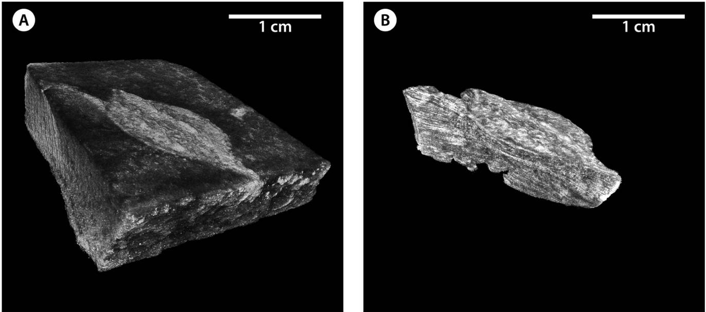
FIG. 5.—X-Ray Computed Tomography (XRCT) of a Copper Harbor structure. **A)** structure within rock matrix. **B)** Copper Harbor structure with matrix digitally removed, showing three-dimensional morphology and “funnel-shape” at depth. Lighter colors reflect higher average density and/or atomic number.
