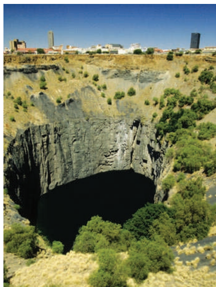
Figure 1 | The Big Hole at Kimberley, South Africa. Here, one hundred years of mining for diamonds, largely by hand pick and shovel, have hollowed out the original funnel-like geometry of the kimberlite eruptive pipe that extends deep below the present water table.
