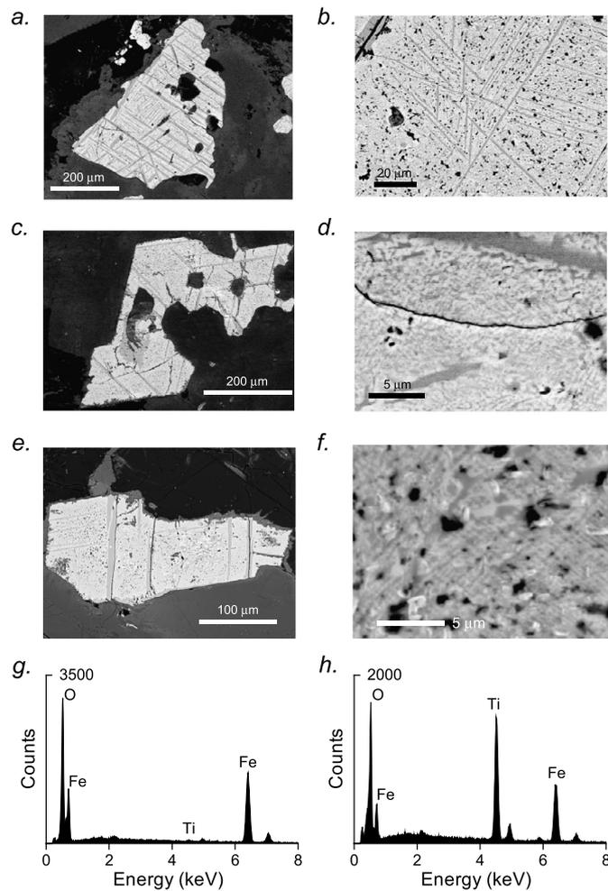
**Fig. 2.** (a, c, e) Examples of backscattered electron images of magnetic grains of the Widgiemooltha dikes showing intergrowths of no/low-Ti (lighter areas) and high-Ti (darker areas) phases. (b, d, f) Examples of finer intergrowth of the no/low- and high-Ti phases within grain interiors (see text). (g, h) Typical energy dispersive spectra from the (g) no/low-Ti and (h) high-Ti phases, interpreted as magnetite and ilmenite/ulvöspinel, respectively (see text).
