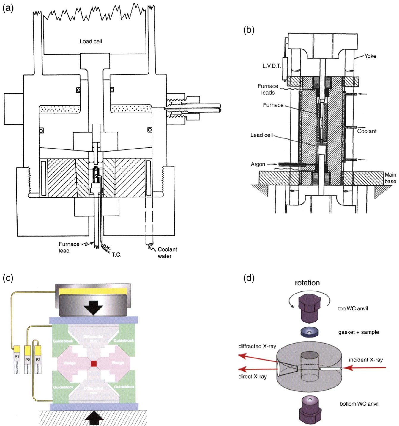
**Fig. 9.** Diagrams of various apparatus for experimental studies of deformation of minerals and rocks. (a) a modified piston-cylinder apparatus (Griggs, 1967). (b) a gas-medium deformation apparatus with an internal load cell (Paterson, 1970). (c) a modified cubic apparatus for deformation studies under high pressures (D-DIA) (Wang et al., 2003). (d) a modified Drickamer apparatus for deformation studies (RDA) (Yamazaki and Karato, 2001).
