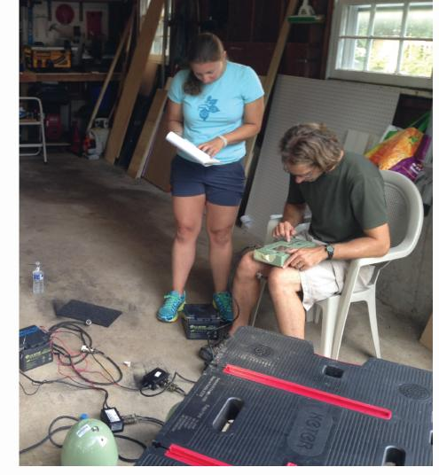
Installation of a broadband seismometer is labor intensive and requires ~4-6 hours of work for a team of ~4 people. Top left: schematic diagram of a station (courtesy of John West). Top right: Photograph of a completed SEISConn station at Fort Hill Farm in Thompson, CT. Left: Equipment being tested by Troy and Meg before deployment in the field, including the datalogger/digitizer, battery, solar panels, and the sensor.
