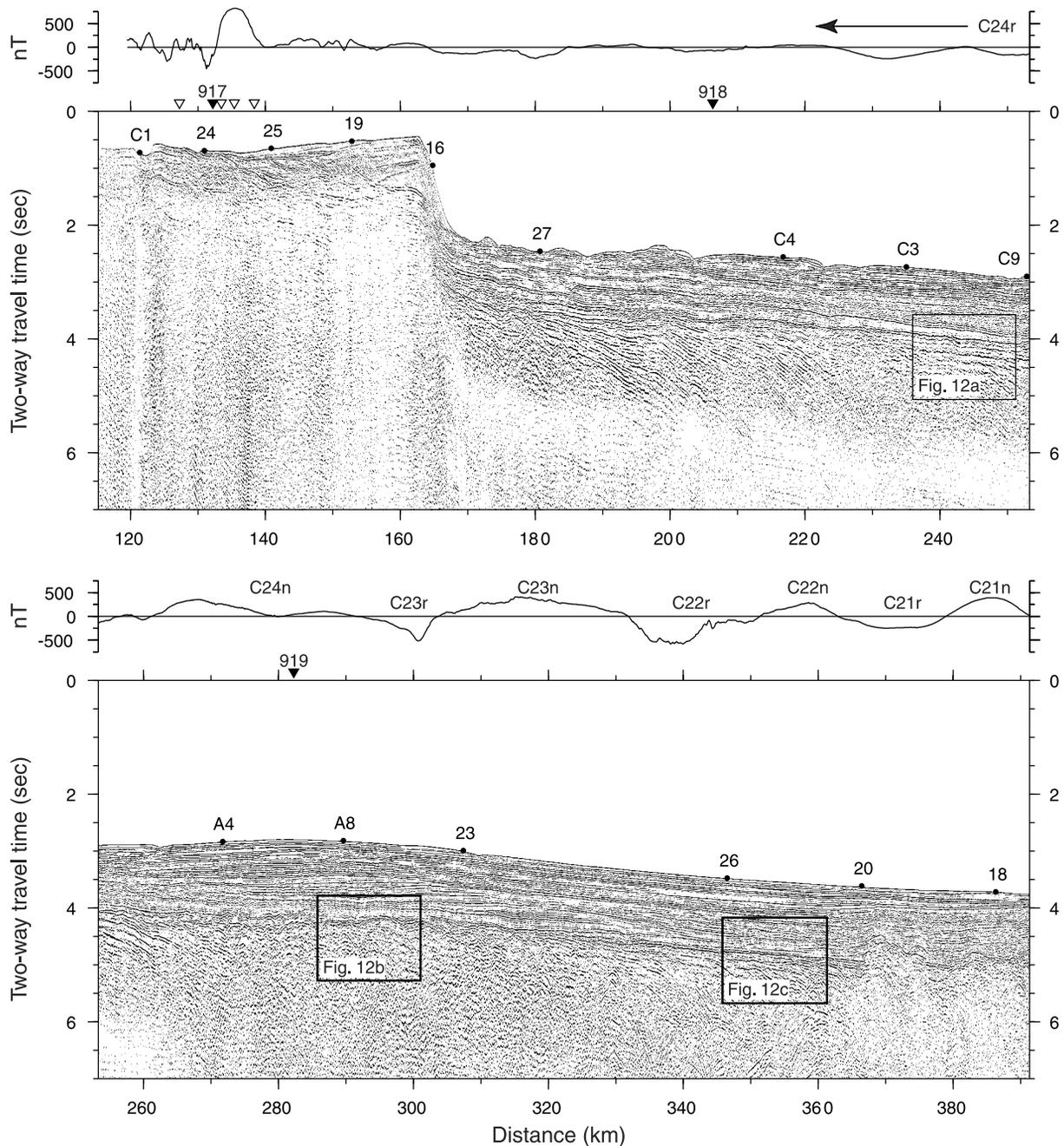
**Figure 3.** Uninterpreted MCS data from SIGMA T-III. See text for data processing information. Dots are ocean bottom stations: USGS OBSs are designated with alpha-numeric labels and WHOI OBHs are designated with numeric only labels. Triangles are ODP Leg 152 and Leg 163 drilling sites. Unlabeled open symbols are Sites 989, 916, 990/915, and 914 from left to right. Magnetic anomaly is from the shipboard magnetometer and interpreted spreading anomalies are labeled.
