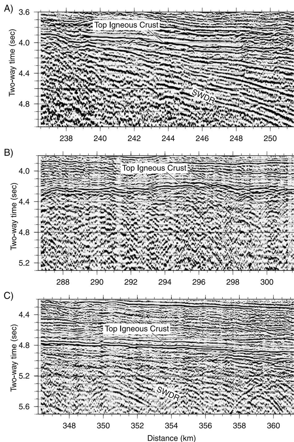
**Figure 12.** Details of seismic reflection data showing the different morphological zones discussed in the text. (a) Subaerially extruded basalts from the main seaward dipping reflector sequence. (b) Shallow marine extrusions. (c) Deep marine extrusions that generate long linear sheet flows and seaward dipping reflectors.
