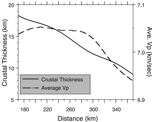
**Figure 9.** Crustal thickness and average velocity as a function of distance along the transect from km 170 (approximate continent-ocean boundary) to the end of line. Crustal thickness decreases nearly linearly along the profile, while the average seismic velocity is constant for the first half of the profile before decreasing toward more normal oceanic velocities.
