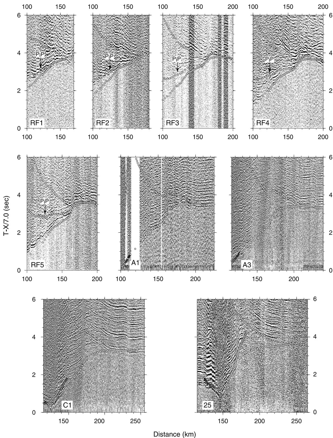
**Figure 5.** Compilation of all wide-angle record sections used in constraining crustal velocity structure along SIGMA T-III. Plots labeled RFx are the REFTEK land stations and the mid crustal reflection is labeled  $P_iP$  on these plots (see text). White dots are calculated travel time arrivals from 2-D ray tracing based on work by Zelt and Smith [1992]. Calculated travel times are for all rays, not just those constrained by travel time picks. Only arrivals from igneous basement are shown.
