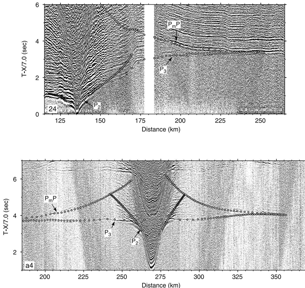
**Figure 4.** Large-scale plots of representative wide-angle record sections. OBH 24 from on the shelf, and OBS A4 from the deeper ocean basin are shown. White dots are calculated travel time arrivals from 2-D ray tracing based on work by *Zelt and Smith* [1992]. Calculated travel times are for all rays, not just those constrained by travel time picks. Only arrivals from igneous basement are shown.
