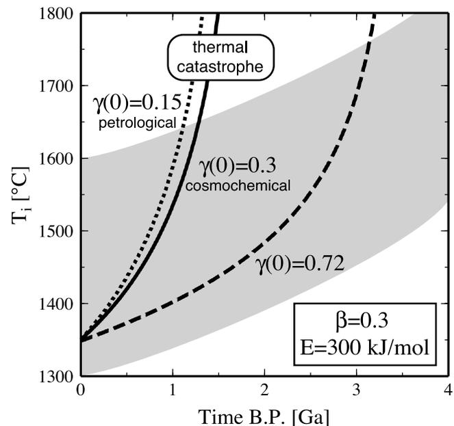
**Figure 2.** Thermal evolution modeling with conventional heat flux scaling of equation (11). The activation energy is set to 300 kJ/mol. Three present-day Urey ratios are used: 0.15 (petrological, dotted), 0.3 (cosmochemical, solid), and 0.72 (superchondritic, dashed). Gray shading denotes the range of potential temperatures recorded in MORB-like suites including greenstone belts and ophiolite suites Figure 5 [Abbott *et al.*, 1994, their Figure 5].
